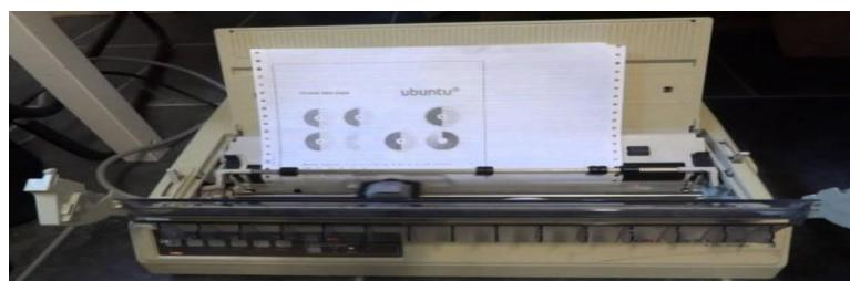
**Fig.13 Dot Matrix Printer**
